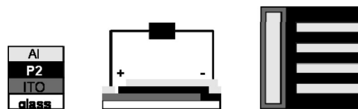
Figure 11. Lateral and top view of a single layer OLED of P2 .
